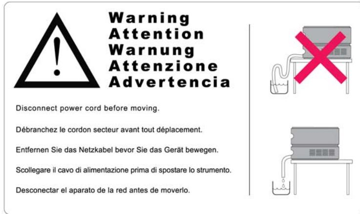
**Figure 14** Warning label (illustration for correct waste tubing)
