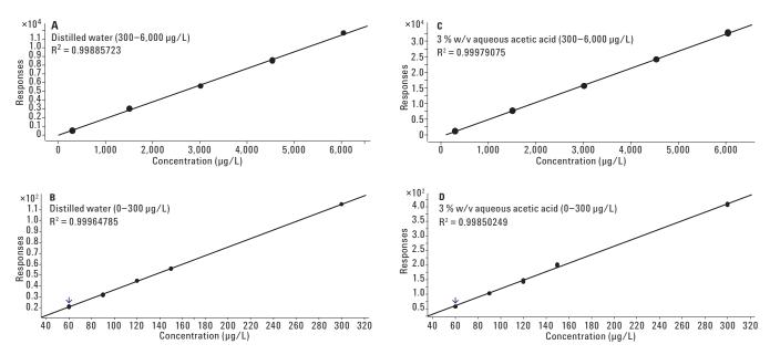
Figure 1. Calibration curves of Bisphenol A. A) distilled water simulant (300–6,000 μg/L), B) distilled water simulant (0–300 μg/L), C) 3 % w/v aqueous acetic acid simulant (300–6,000 μg/L), and D) 3 % w/v aqueous acetic acid simulant (0–300 μg/L).
