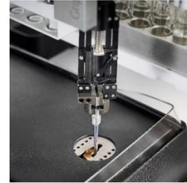
The probe is thermally desorbed and the vapours transferred to the focusing trap.
