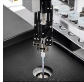
The probe is removed from the vial and a wash/dry station removes the residual sample matrix.
