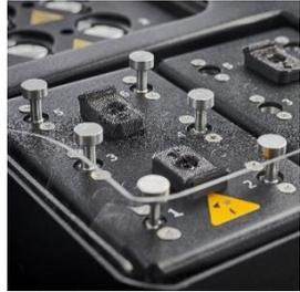
Probe storage keeps probes clean and ensures conditioned probes are ready to be used.
