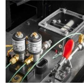
The trap is thermally desorbed at up to 100°C/s in inject the sample into the GC-MS system.
