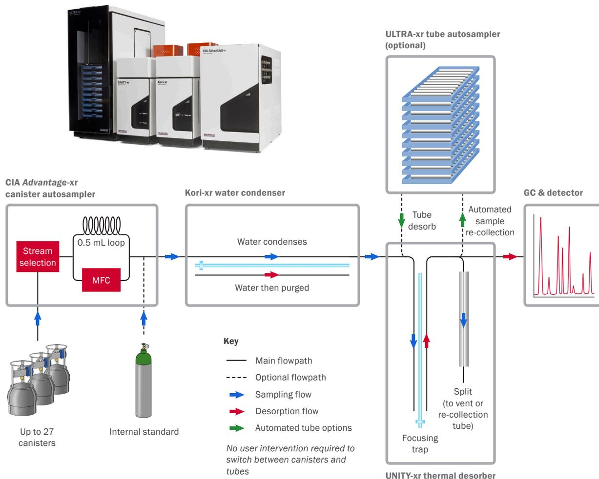
**The modular nature of CIA Advantage-xr systems** means that options for tube analysis and sample re-collection are easily configured – complementing the capability for addition of internal standards inherent to every instrument.
