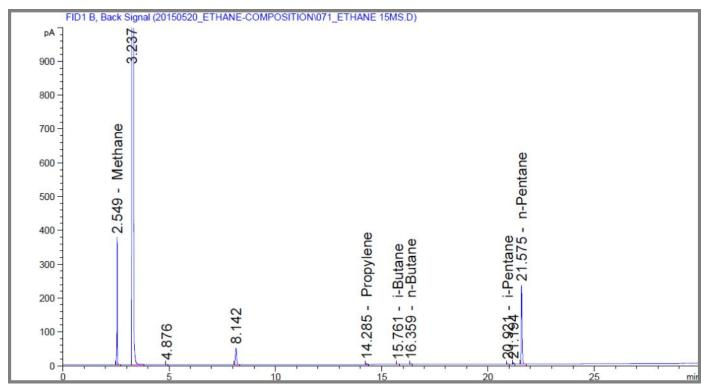
Figure Four: Chromatogram of the LGI analysis of light hydrocarbons of liquid Ethane
