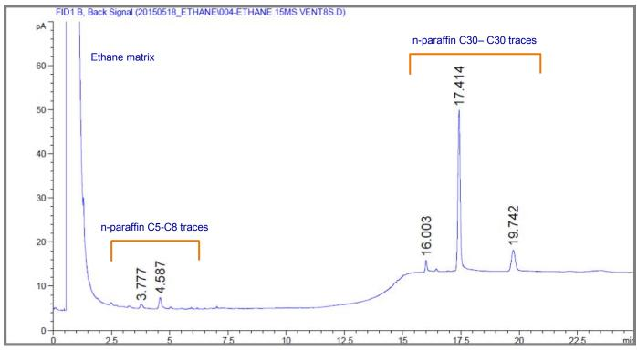
Figure Three: Chromatogram of the LGI analysis of residue in liquid Ethane
