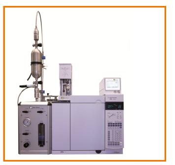
Figure One: the DVLS Liquefied Gas Injector
