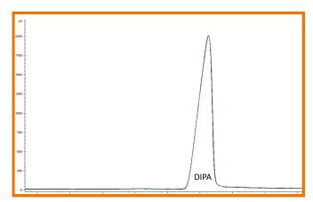
Figure Four: Overlay of three chromatograms of 125 ppm DIPA
