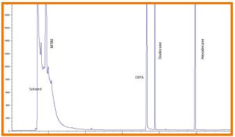
Figure Three: Chromatogram of 125 ppm DIPA in Pentane
