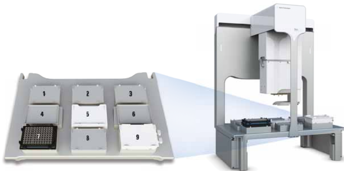
Figure 15. The Agilent Bravo Automated Liquid Handling Platform and Bravo deck layout for a CYP450 assay, with one Orbital Shaking Station (location 8). One stack of five microplates (location 7), three reservoirs (locations 1–3), and three tip boxes (locations 4–6) are placed manually on the deck before the protocol is started. (See Agilent publication 5990-3550EN.)
