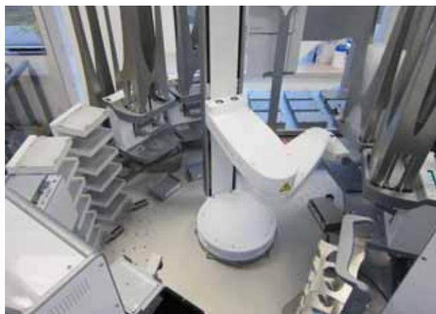
Figure 16. A customized BioCel automation solution, consisting of a Bravo Platform, PlateLoc® Sealer, Hotel and LabWare Stackers, and a DDR robot.
