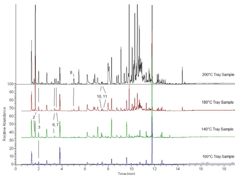
Figure 1 – Overlay of the Total Ion Current of the PET Tray Samples at 100°C (212°F), 140°C (284°F), 180°C (356°F) and 200°C (392°F) Dynamic Sample Temperatures.
