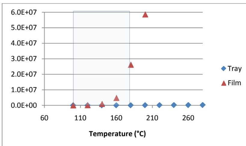
Figure 4: Temperature Profile Plot of the Chloromethane Peak Area for the Tray Sample (blue diamond) and the Film Sample (red triangle). The grey box indicates the cooking temperature range from 100°C (212°F, boiling water) to the manufacturer's upper oven limit of 177°C (350°F)
