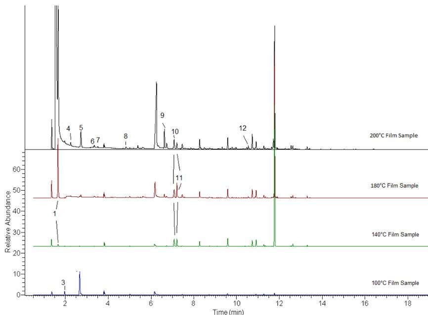
Figure 3: Overlay of the Total Ion Current of the Film Samples at 100°C (212°F), 140°C (284°F), 180°C (356°F) and 200°C (392°F) Dynamic Sample Temperatures.
