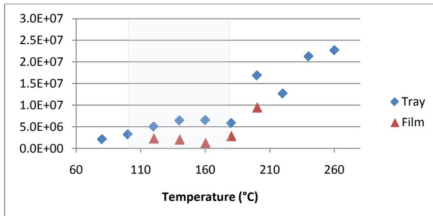
Figure 2 – Temperature Profile Plot of the Acetaldehyde Peak Area for the Tray Sample (blue diamond) and the Film Sample (red triangle). The grey box indicates the cooking temperature range from 100°C (212°F, boiling water) to the manufacturer's upper oven limit of 177°C (350°F)
