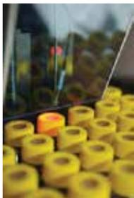
When programmed for soil samples, the Centurion's arm will go to the sample position and look to see if a sample vial is in the tray. The Centurion uses a fiber optic sensor for this instead of a mechanical switch that can be unreliable. Once detected, the gripper will pick up the vial and move it to the heated soil station.
