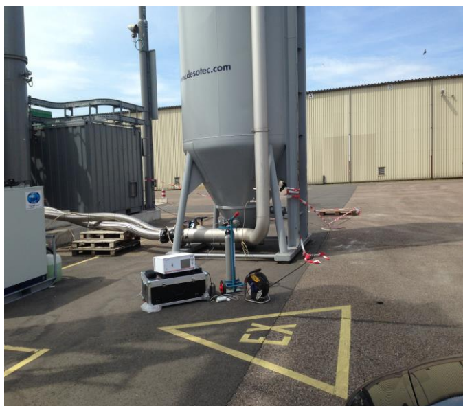
Figure 7: GC-IMS SILOX on-site. The instrument precisely quantifies individual siloxanes species, L2-L5 same as D3-D5, calculates 'total silicon' and 'total silica' and by this allows to take a reliable decision on-site. Besides a flexible spot-to-spot measurement using its one-click operation it even enables a continuous and remote online monitoring to test for the pipe gas same as for a potential filter breakthrough while sampling and quantifying the siloxanes automatically in user defined intervals.
