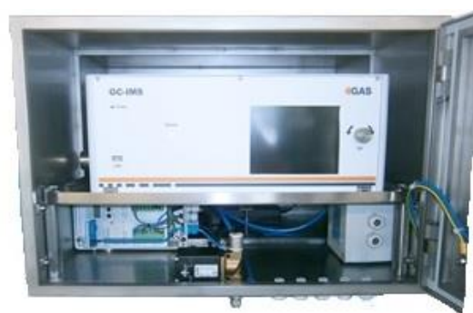
Figure 6: GC-IMS instrument for monitoring of TICs in chemical plants embedded into a pressurized enclosure system. The pressurized enclosure system ensures safety class Ex II 2 G Ex px II T4 (German Explosion Protection Ordinance).
