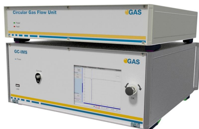
Figure 4: Portable measurement system - CGFU (Circular Gas Flow Unit) coupled to a GC-IMS. For full performance the system only needs power supply.
