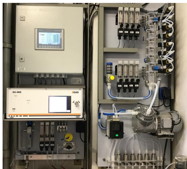
Figure 5: GC-IMS on-site integrated into process measuring and control technology system of Bilfinger Maintenance GmbH.
