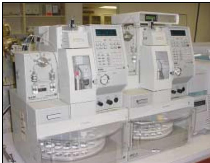
Figure 9. OI Analytical Dual Purge-and-Trap System Using the PT Express and SAM
