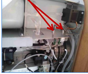
Unscrew the 2 screws with Allen key
