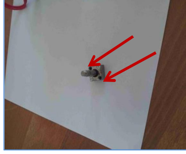
•Unscrew the two screws at the top right and bottom left to open the valve
