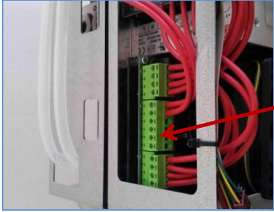
Disconnect the terminal block central green
