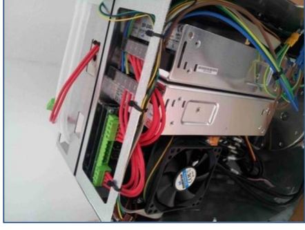
Cut the three fixing wires
