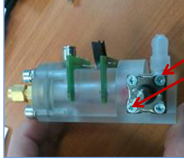
•Unscrew the two screws at the top left and bottom right and remove the valve
