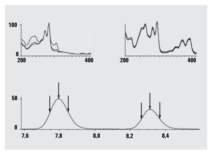
Figure 4 Peak-Purity Check by Overlaying Spectra
