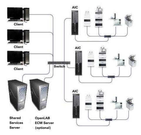
Figure 1 Distributed System Configuration
