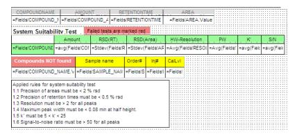
Figure 91 System suitability test layout in the Impurity Profiling template
