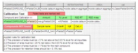
Figure 92 Calibration test layout in the *Impurity Profiling* template
