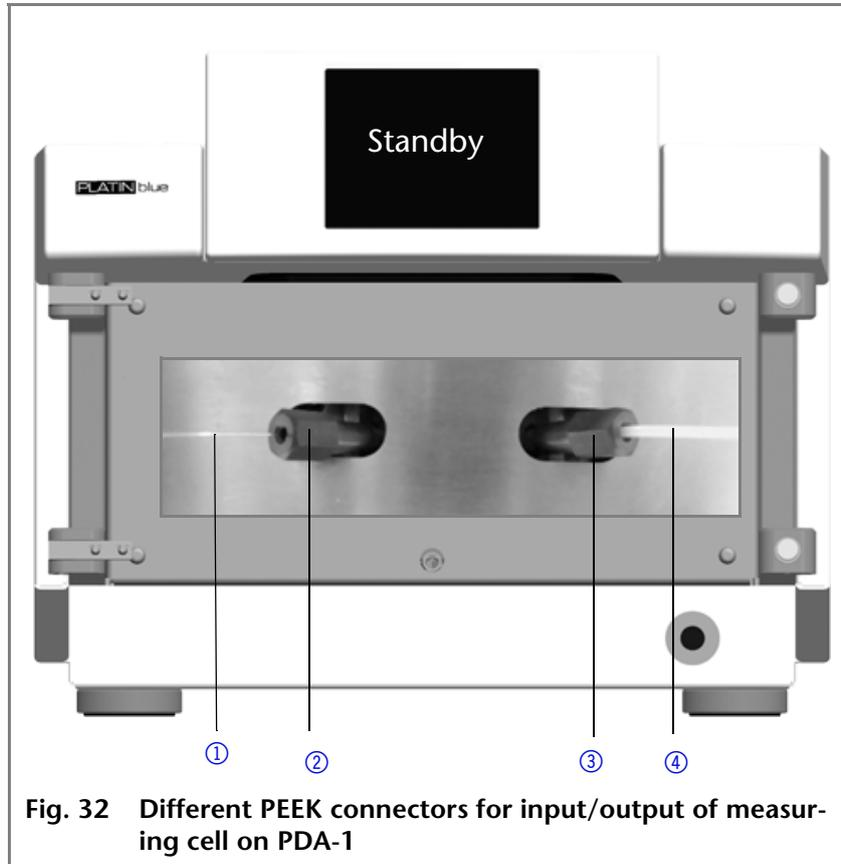
Fig. 32 Different PEEK connectors for input/output of measuring cell on PDA-1
