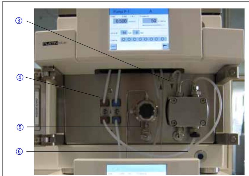
HPG pump P-1 with HPG mixing chamber ⑦, pressure sensor, venting valve and pump head
