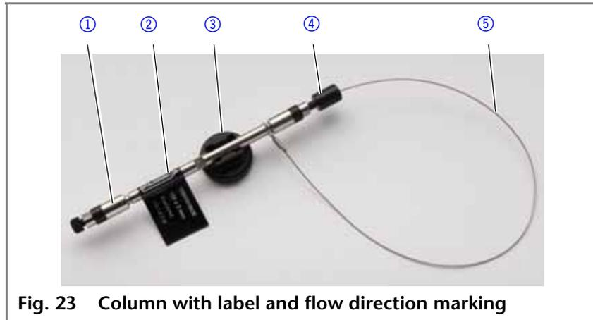
Fig. 23 Column with label and flow direction marking
