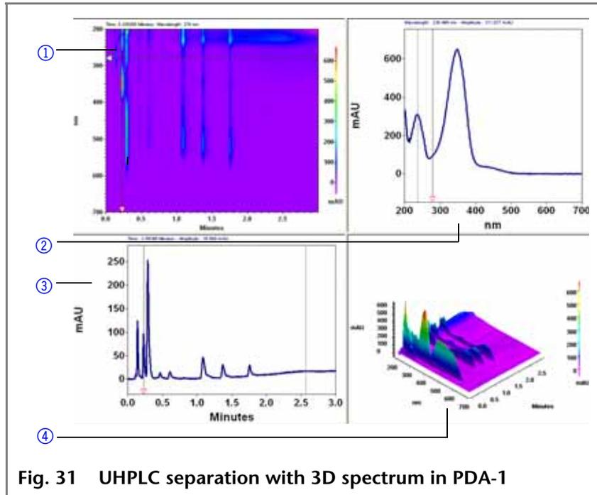
**Fig. 31** UHPLC separation with 3D spectrum in PDA-1
