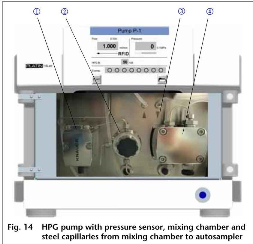
Fig. 14 HPG pump with pressure sensor, mixing chamber and steel capillaries from mixing chamber to autosampler
