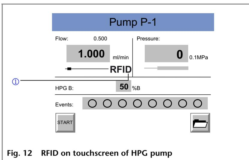
Fig. 12 RFID on touchscreen of HPG pump
