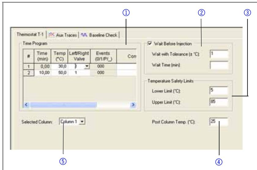
**Fig. 80** Method window ('*Instrument Setup*' window) of the T-1 column thermostat
