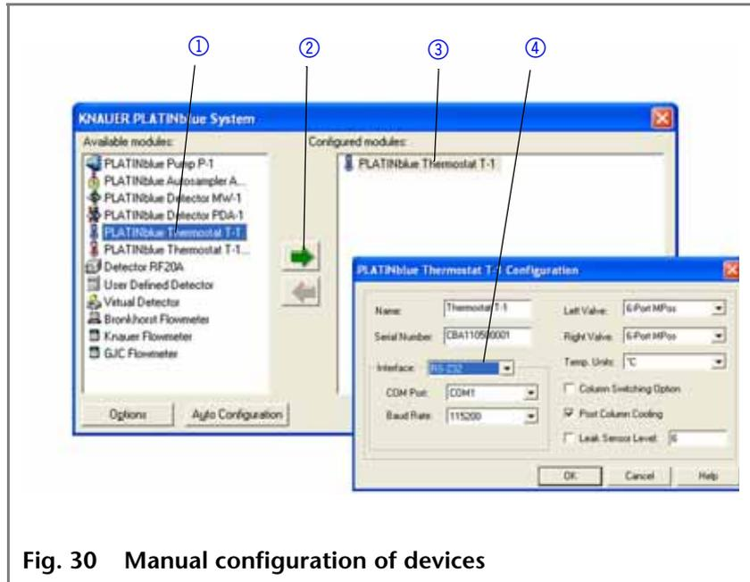
**Fig. 30** Manual configuration of devices
