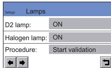
**Fig. 63** Setting the detector lamps
