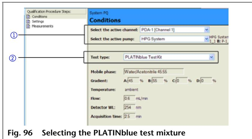
Fig. 96 Selecting the PLATINblue test mixture
