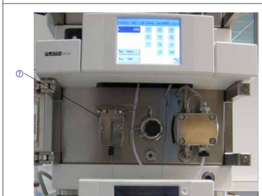
Autosampler AS-1 ① with interior retractable door; Injection valve, see S. 52
