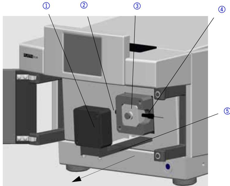
**Fig. 108** MW-1 detector with flow cell, capillary connections and assembly carriage
