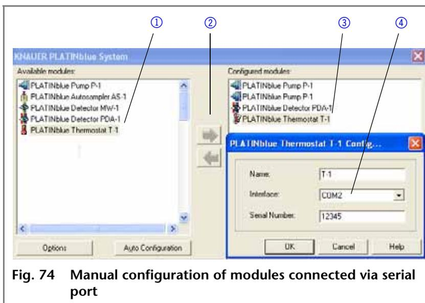
**Fig. 74** Manual configuration of modules connected via serial port
