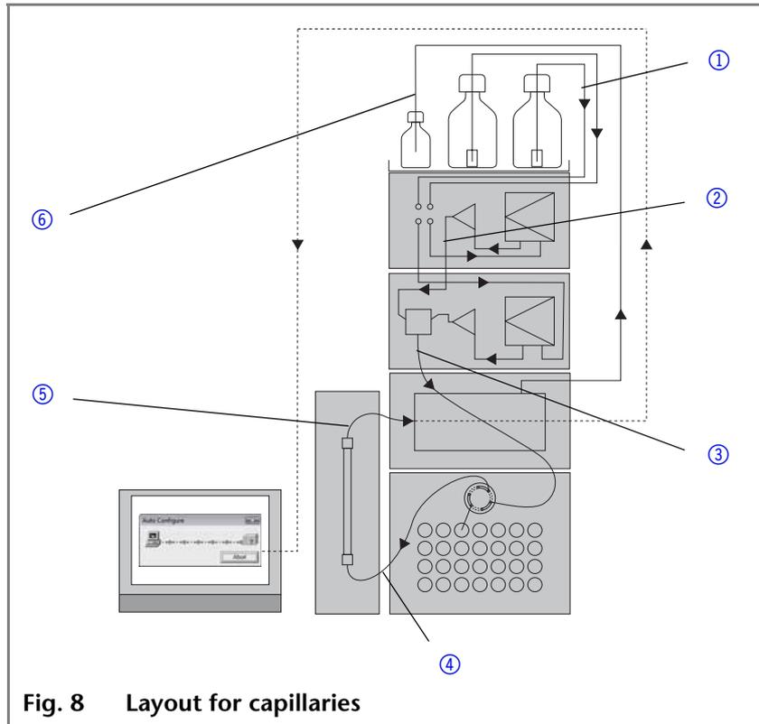
Fig. 8 Layout for capillaries
