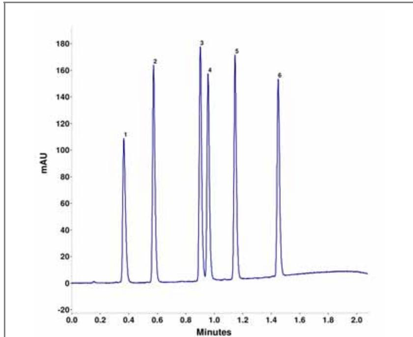
**Fig. 1** UHPLC separation of steroids in less than two minutes
