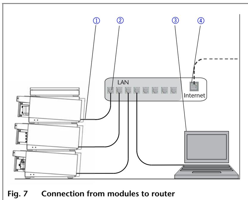
Fig. 7 Connection from modules to router
