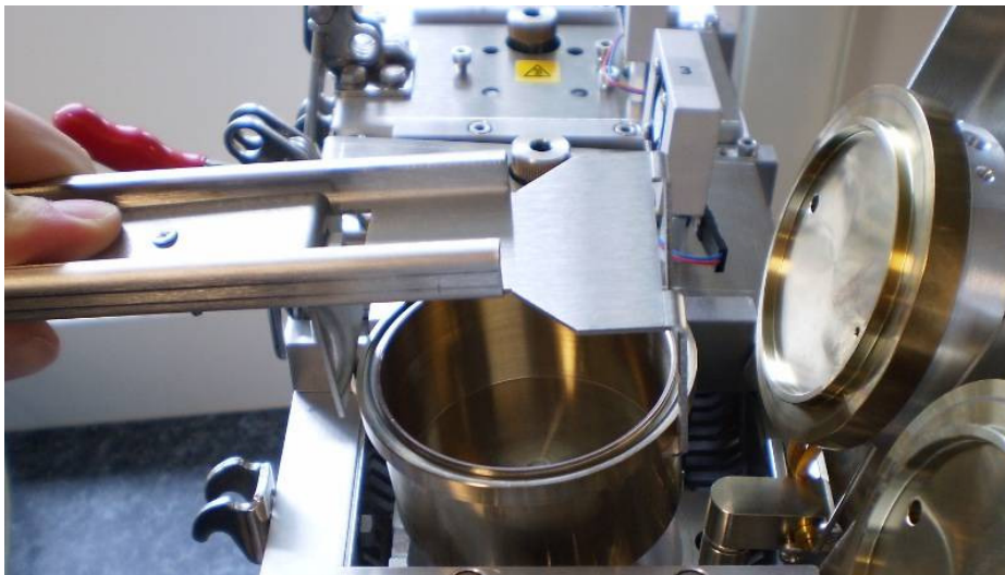
Figure 6: Removing a hot pot with the removal tool
