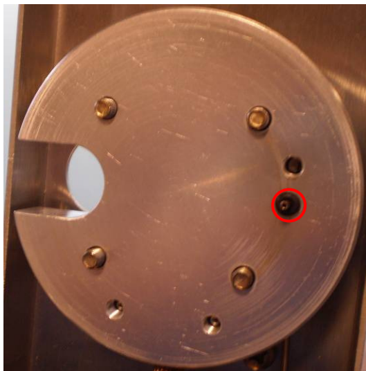
Figure 7: Position of O-ring for removal
