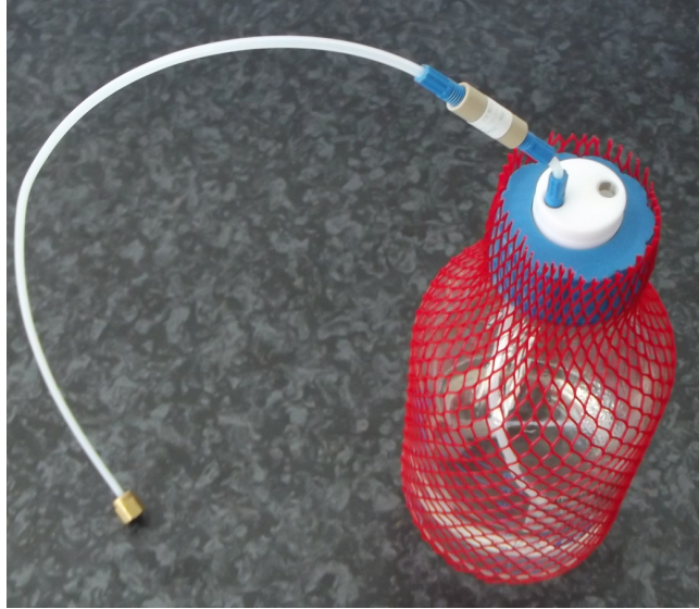
Figure 2: Connecting the Input Assy to the Humidifier Bottle. (NB – length of Tube is shortened to 200mm here.)
