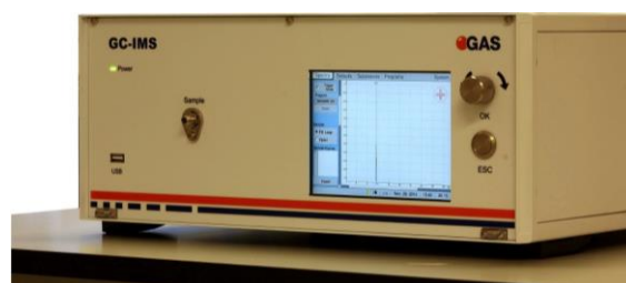
Figure 4: GC-IMS instrument for monitoring of TICs in chemical plants.
