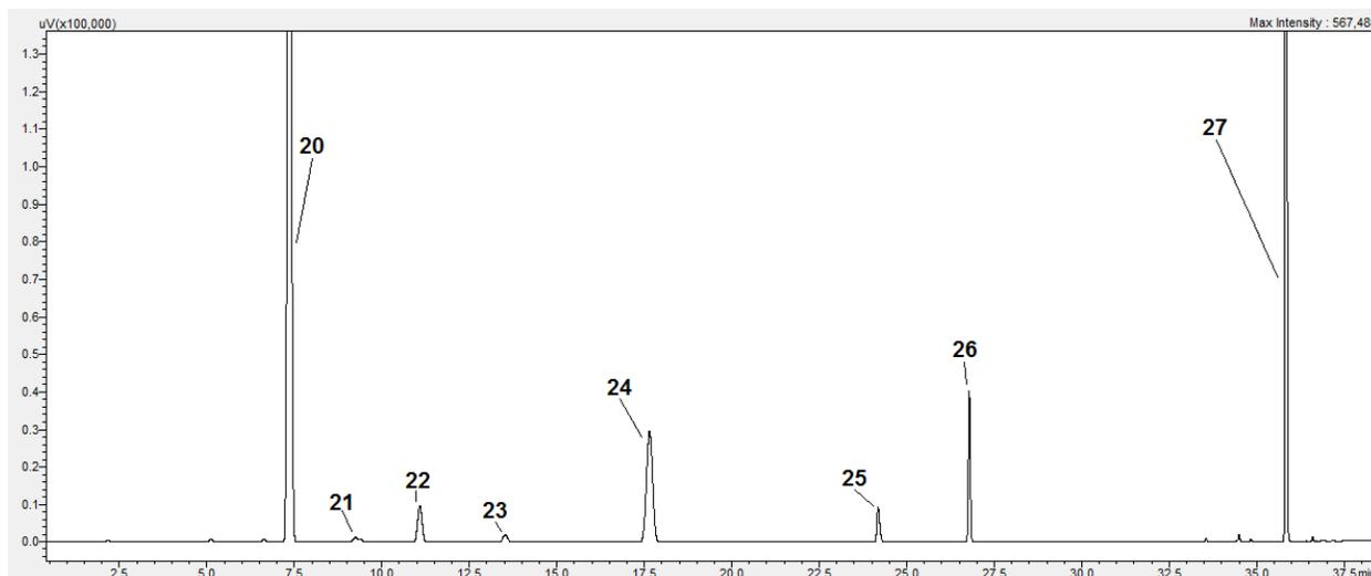
Figure 3: Chromatogram of a Class 2B Standard (data for corresponding peaks can be found in Table 8)
