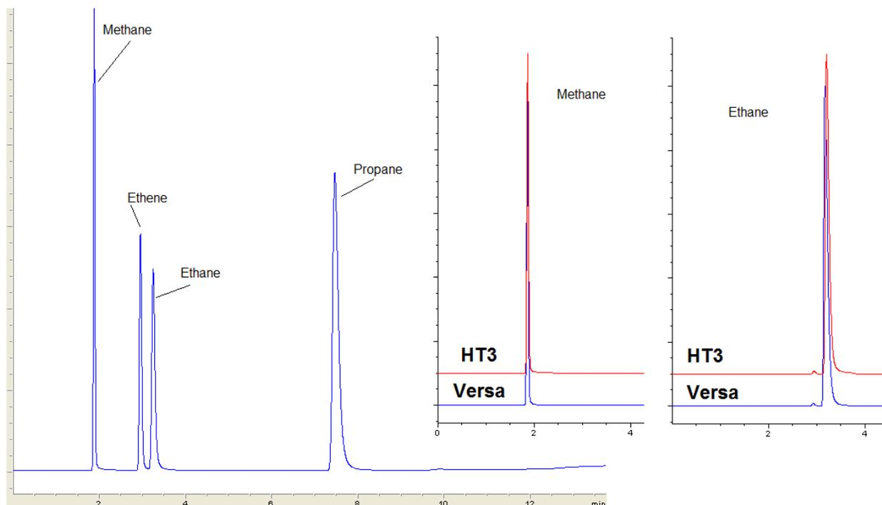
Figure 1: Gas Chromatogram Comparison of Methane and Ethane between the HT3 and the Versa and the Chromatogram of the Four Gases.
