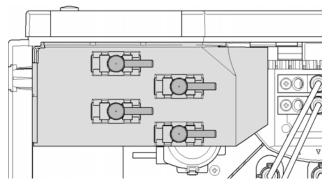
**5** Connect the solvent tubes from the bottle head assemblies to the inlet connectors A1, A2, B1 and B2 of the solvent selection valves. Use the brown bottle for the aqueous solvent (usually channel A1).
