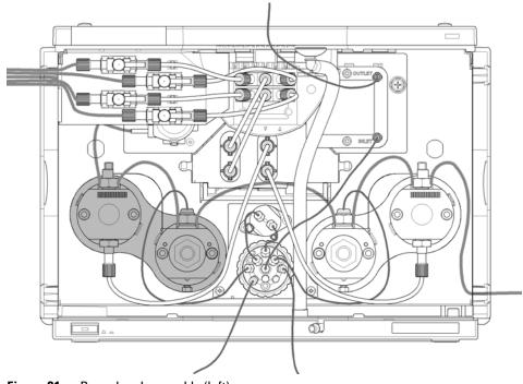
Figure 21 Pump head assembly (left)
