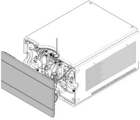
Figure 11 Removing the Front Cover
