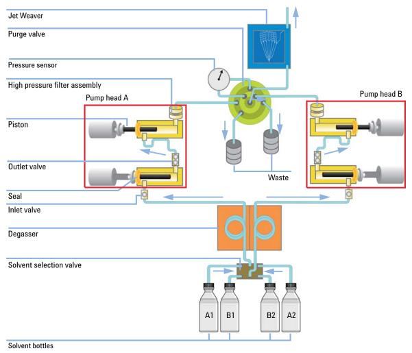
**Figure 1** The hydraulic path
