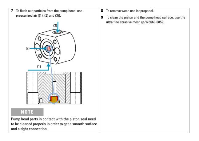
**Disassembling the Secondary Pump Head**
