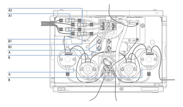
Flow connections to the pump
