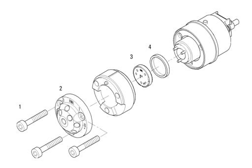
Figure 31 Purge valve parts
