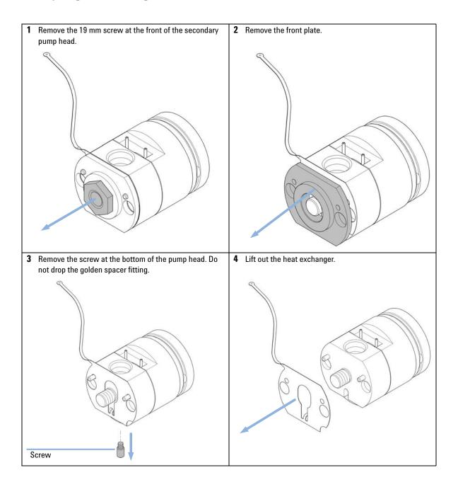
**Replacing the Heat Exchanger**
