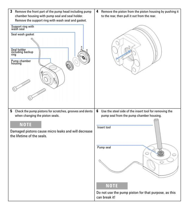
**Disassembling the Secondary Pump Head**
