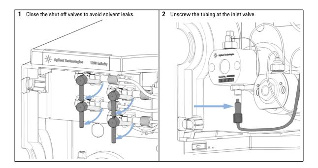
**Replacing the Inlet valve**
