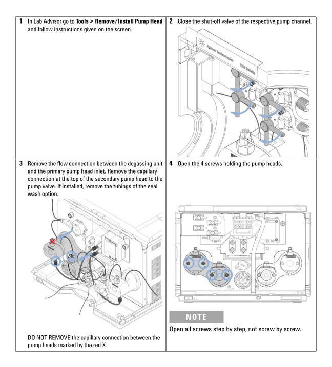
**Replacing the Pump Heads**
