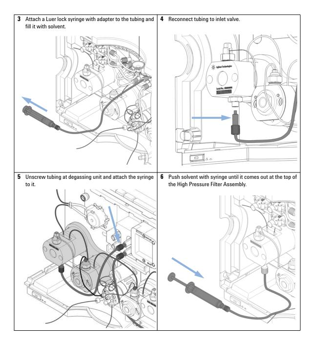
**Releasing a Stuck Inlet Valve**
