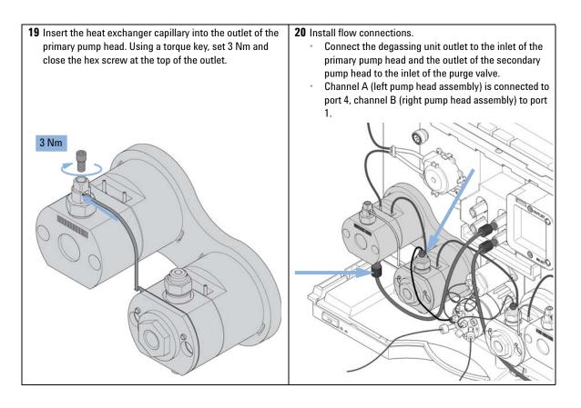
**Replacing the Purge Valve Head**
