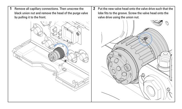
**Replacing the Purge Valve Head**
