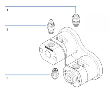
Figure 26 Pump head assembly parts
