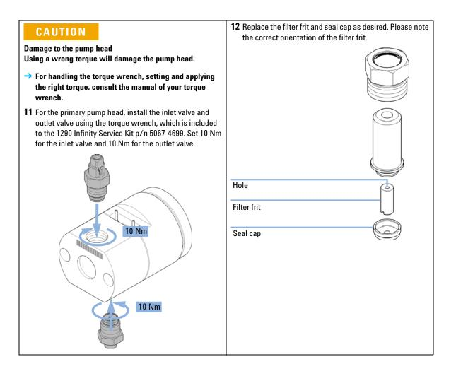
**Assembling the Pump Head**
