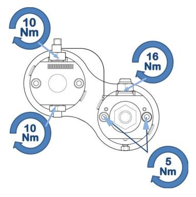
Figure 20 Overview of torques for pump head procedures
