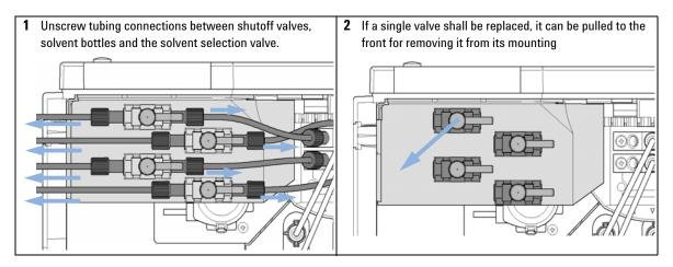
**Replacing the Shutoff Valve Panel**
