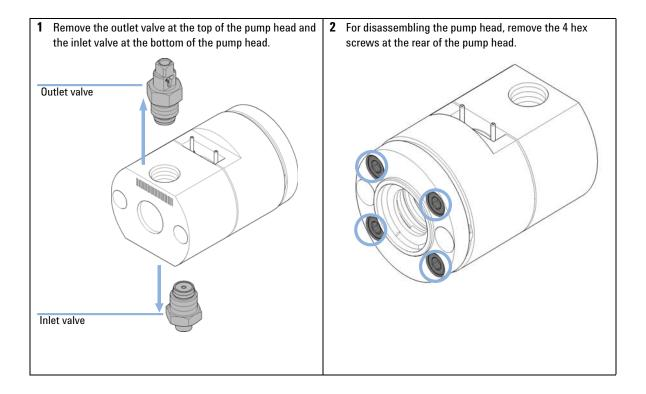
**Disassembling the Primary Pump Head**
