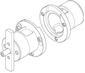
Figure 35 Pump head alignment tool
