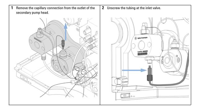
**Releasing a Stuck Inlet Valve**
