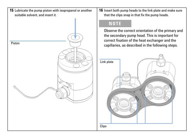
**Assembling the Pump Head**
