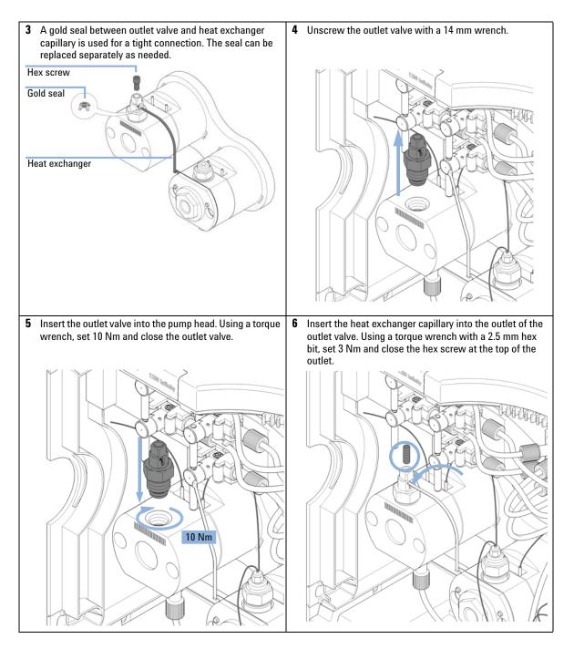
Replacing the Outlet Valve
