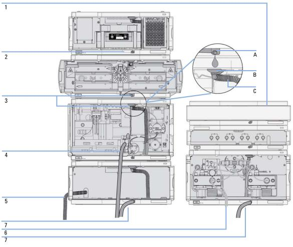
**Figure 7** Leak and waste handling (overview - typical stack configuration as an example)
