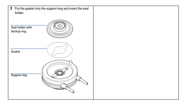
Assembling the Pump Head
