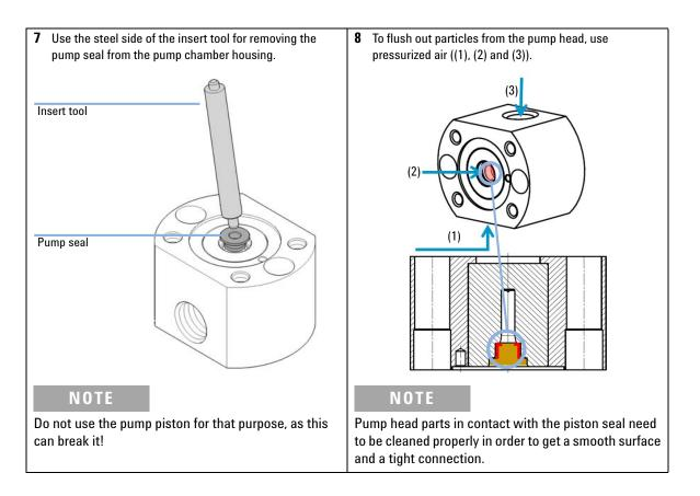
**Disassembling the Primary Pump Head**
