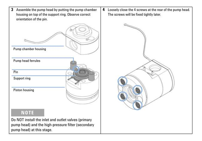
**Assembling the Pump Head**
