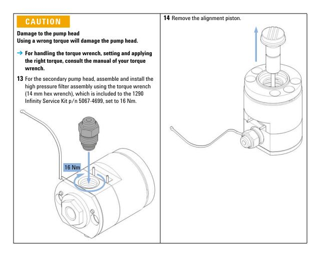
**Assembling the Pump Head**
