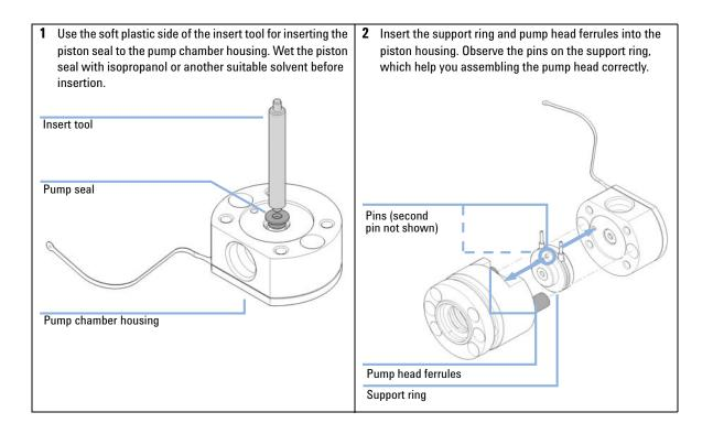
**Assembling the Pump Head**
