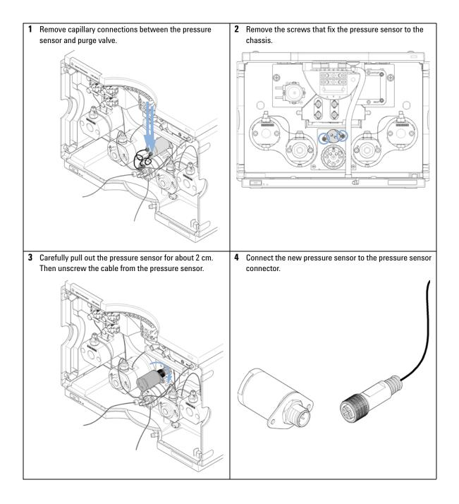
**Replacing the Pressure Sensor**
