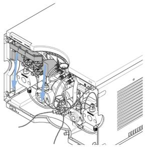
**3** Remove the shutoff valve panel by pulling it downwards
