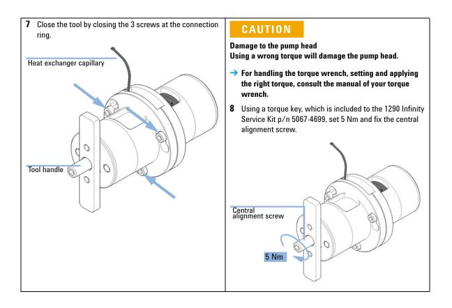
**Assembling the Pump Head**
