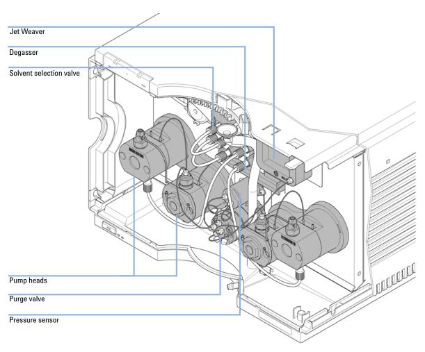
The pump is shipped with tubing and capillary connections installed between solvent selection valve, degassing unit, pump heads, pressure sensor, purge valve and Jet Weaver. This section describes the installation of additional flow connections.
