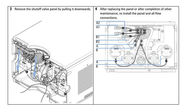
**Replacing the Pressure Sensor**
