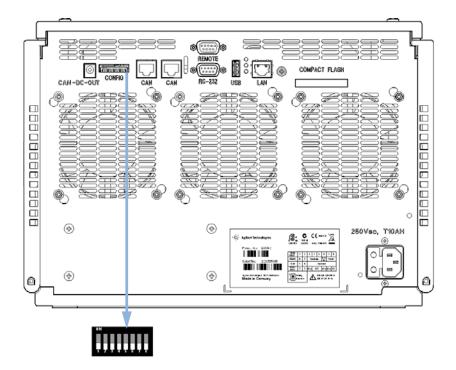
The configuration switch can be accessed at the rear of the module.
