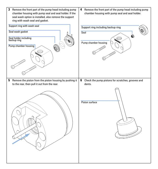
**Disassembling the Primary Pump Head**
