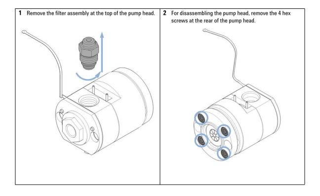
**Disassembling the Secondary Pump Head**
