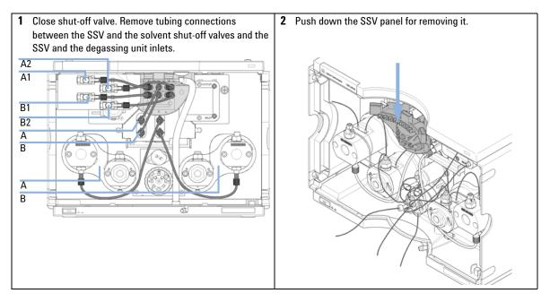
**Replacing the Solvent Selection Valve (SSV)**
