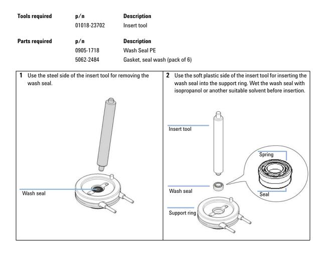
**Replacing Wash Seal and Gasket**
