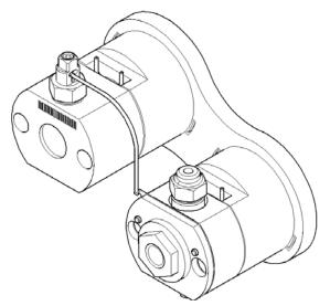
Figure 25 Pump head assembly (left) with seal wash option
