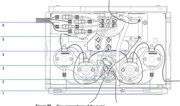
Figure 23 Flow connections of the pump
