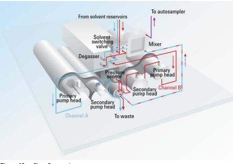
Figure 19 Flow Connections
