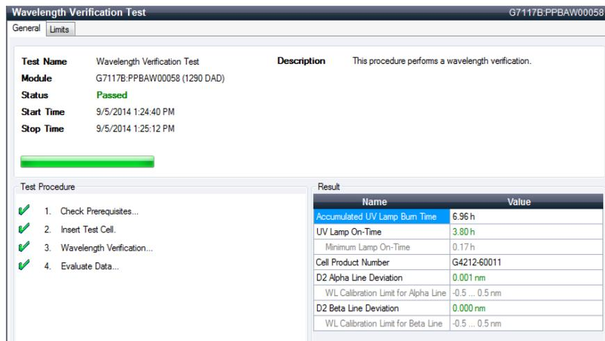
**Wavelength Verification Test** G7117B:PPBAW00058
