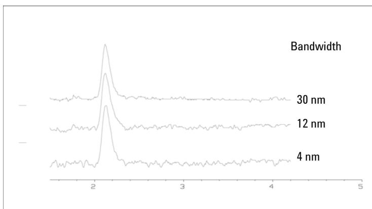
**Figure 20** Influence of Bandwidth on Signal and Noise
