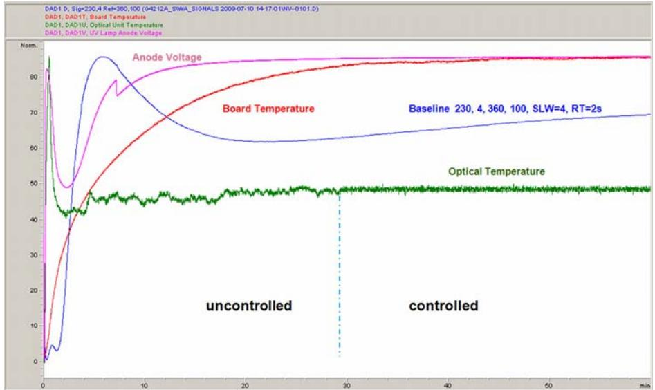
Figure 29 Detector Warm-up – 1<sup>st</sup> hour
