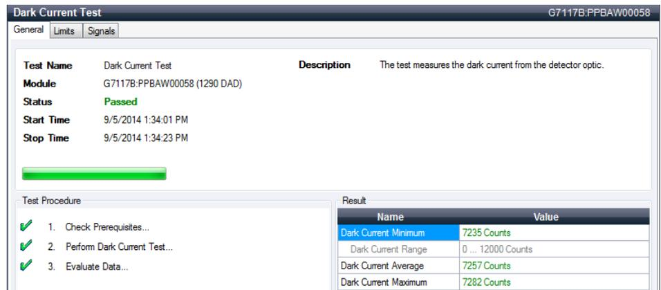
**Figure 47** Dark Current Test – Results
