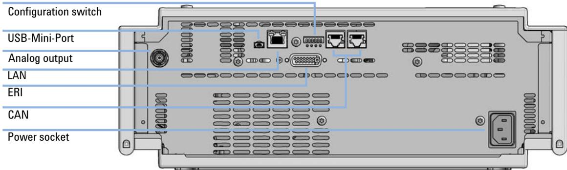
**Figure 51** Rear view of detector (example shows a G7114A/B VWD) – electrical connections and label
