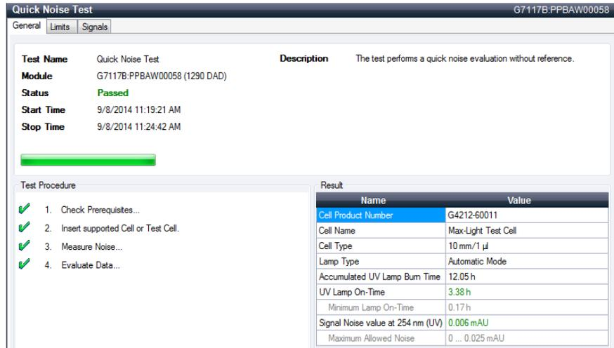
**Figure 37** Quick Noise Test – Results
