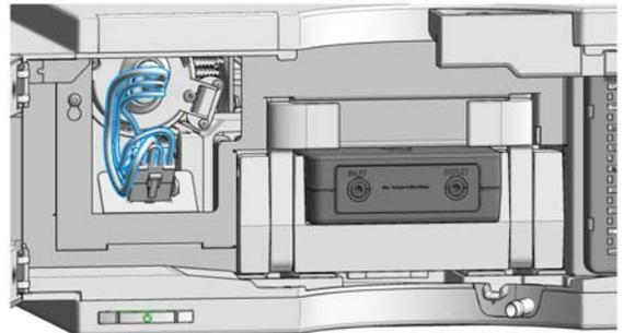
**9** Slide the lamp cover into the top position of the metal front (1.) and press the lamp cover completely in until it clicks (2.).
