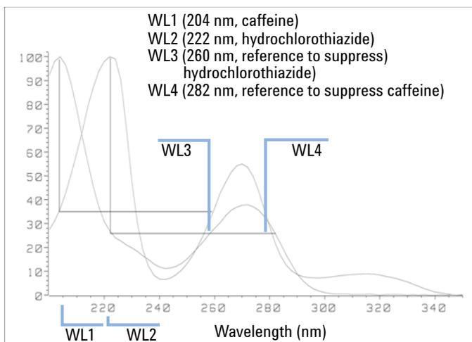
**Figure 24** Wavelength Selection for Peak Suppression
