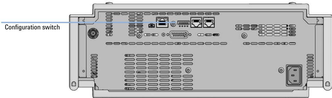
**Figure 53** Location of Configuration switch (example shows a G7114A/B VWD)
