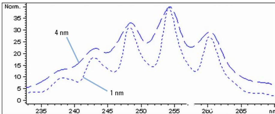
**Figure 22** Benzene at 1 and 4 nm slit width (principle)
