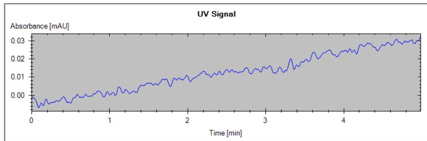
**Figure 38** Quick Noise Test – Signal
