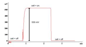
Fig. 2. Measuring output with dummy cell off and on at 5 nA/V, for other settings see Table IV.
