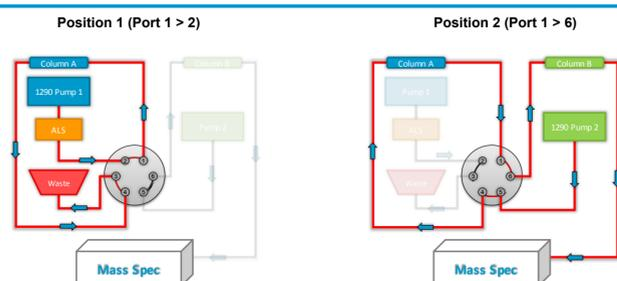
Figure 2. Back-Flush LC configuration for online sample cleanup and heart-cutting
