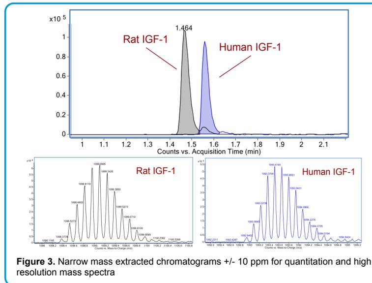
Figure 3. Narrow mass extracted chromatograms +/- 10 ppm for quantitation and high resolution mass spectra
