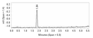
Figure 2. 100 ppb hydrogen sulfide in ethylene.
