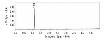
Figure 1. 60 ppb carbonyl sulfide in propylene.
