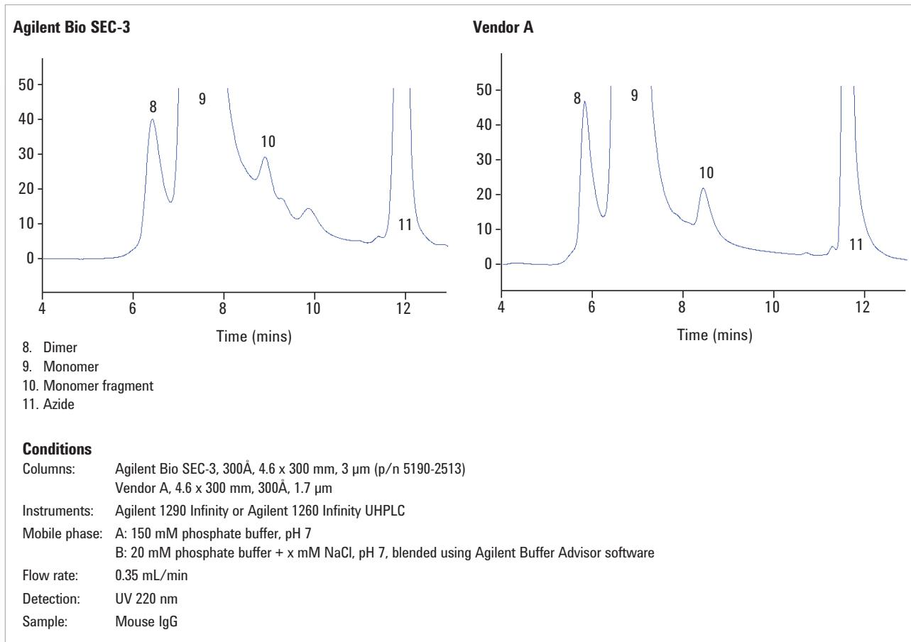
We further evaluated the effect of chemistry and particle size on separation with a polyclonal mouse IgG test mix. The Agilent Bio SEC-3 had the best definition of the fragmentation pattern for the mouse IgG, due to the proprietary hydrophilic coating of the Agilent Bio SEC-3 column, which reduces secondary interactions and improves resolution.
