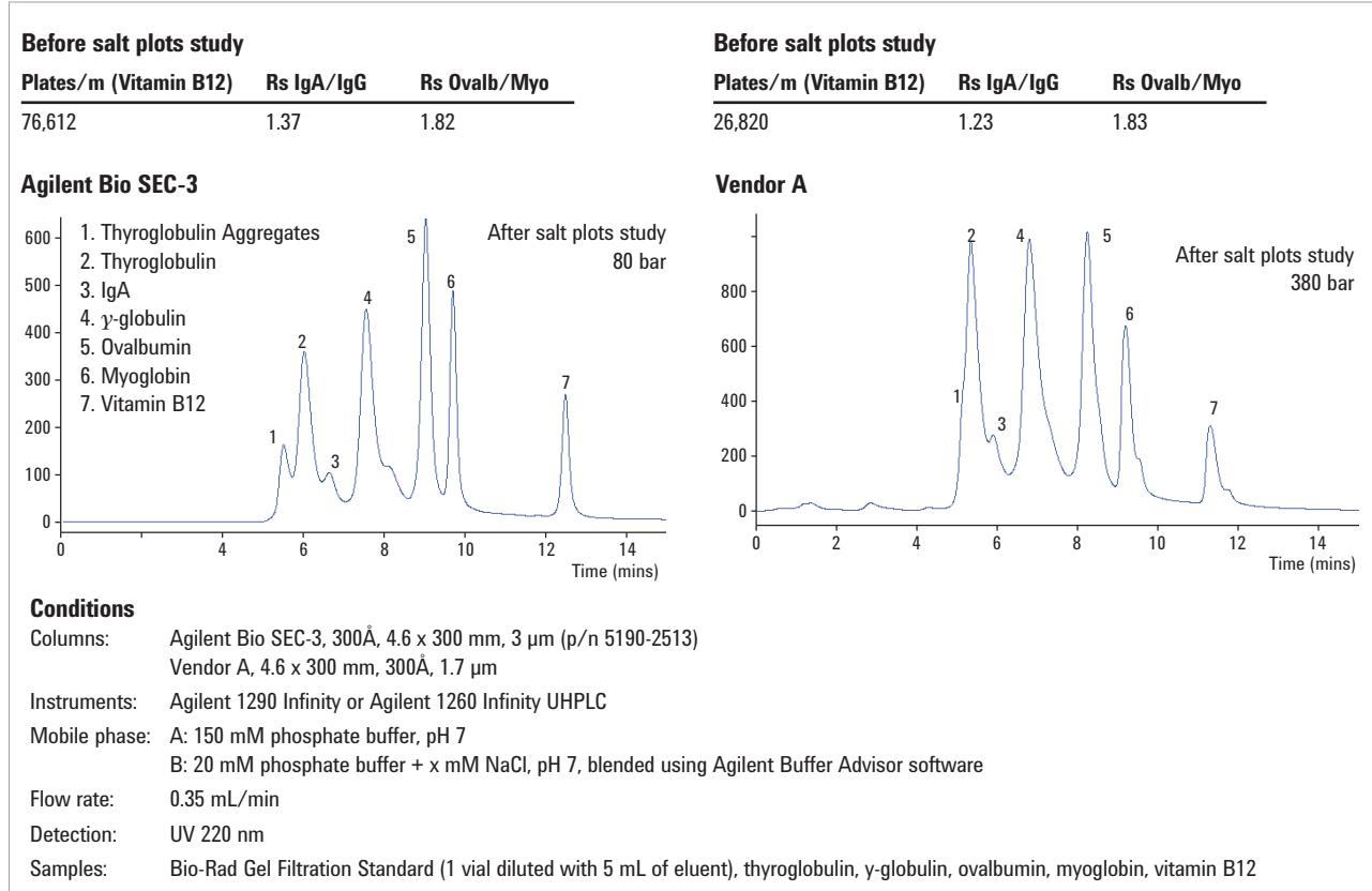
The change in efficiency and resolution of the protein standard separations after completing the evaluations of non-specific interactions using different salt concentrations is evident. The Agilent Bio SEC-3 column is more robust.
