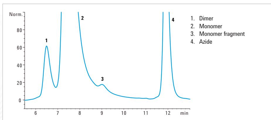
Magnification of the mouse IgG separation using an Agilent Bio SEC-3 300Å column – the best choice for this analysis.
