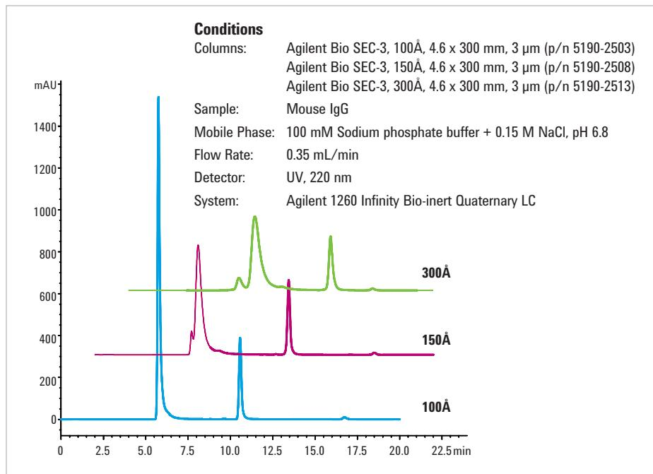
Separation of mouse IgG on Agilent Bio SEC-3 columns with three different pore sizes. Here, resolution increased with pore size: The 100Å pore size column excluded the IgG, so no definition was achieved; partial exclusion with the 150Å, and 300Å columns successfully resolved the monomer and dimer.
