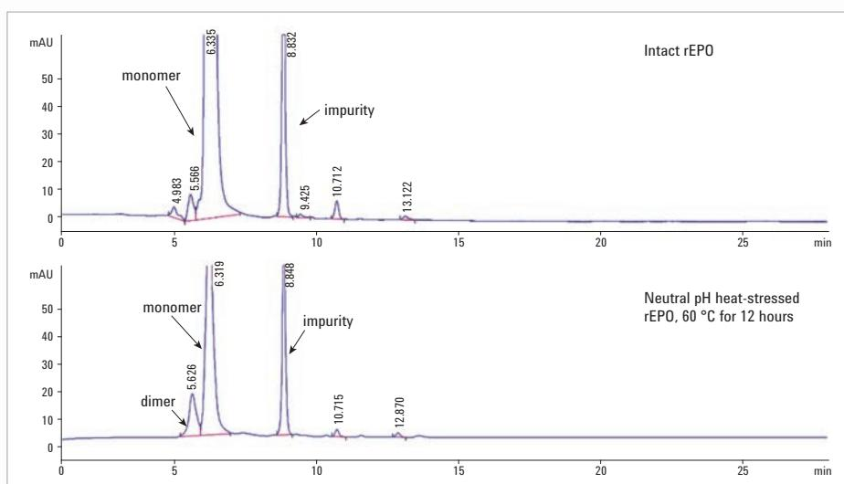
The dimer peak increased to 11%, whereas the monomer peak decreased to 62.5%. Although the reduction was not as severe as with low-pH, heat-stressed rEPO, the data clearly demonstrate that the Bio SEC-3 column successfully resolved different sizes of rEPO impurities and degradation products.
