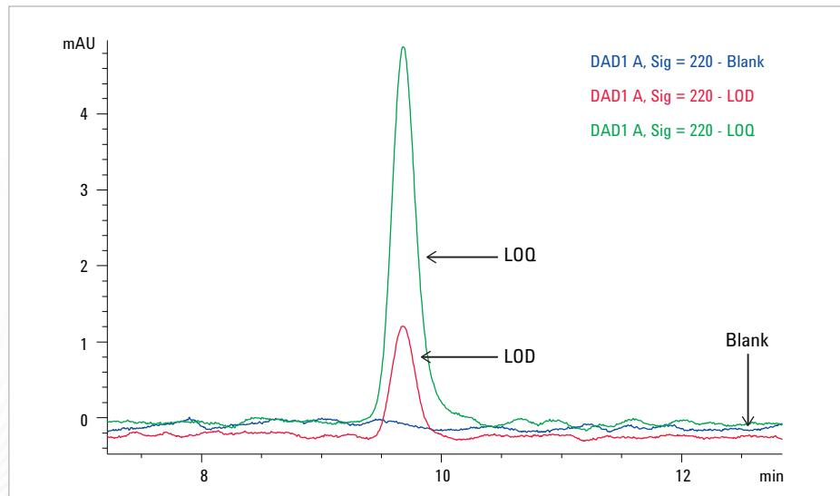
LOD (12.5  $\mu\text{g/mL}$ ) and LOQ (25  $\mu\text{g/mL}$ ) chromatograms of IgG1 overlaid with blank.
