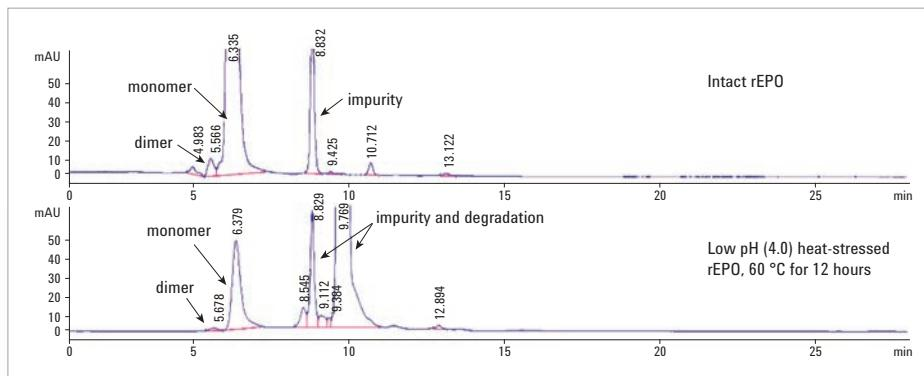
rEPO has limited stability at low pH and high temperature – the monomer peak is reduced in size and peaks due to smaller fragments resolved.
