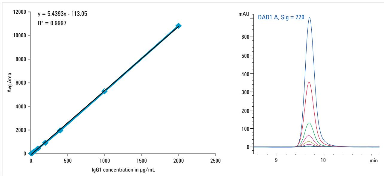
These IgG1 linearity curves were constructed from the LOQ level to the highest concentration of the study. Observed accuracy values of 82 to 112%, representing the range of 100 to 2,000 µg/mL, indicate that the SEC method is quantitative and accurate.
