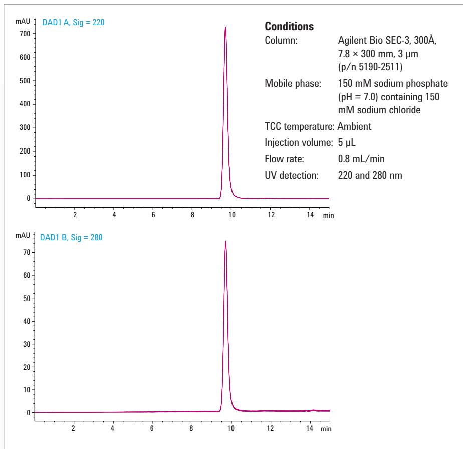
Profile of intact IgG1 on an Agilent Bio SEC-3, 300Å, 7.8 × 300 mm, 3 µm column (overlay of six replicants).
