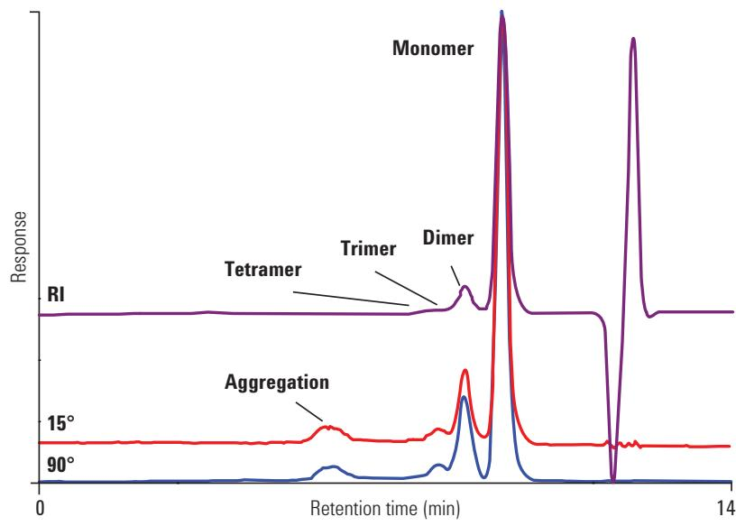
Overlay of the differential refractive index and dual-angle light scattering data showing monomer, dimer, trimer, and aggregation peaks. These results illustrate the power of light scattering, coupled with SEC, in protein characterization.
