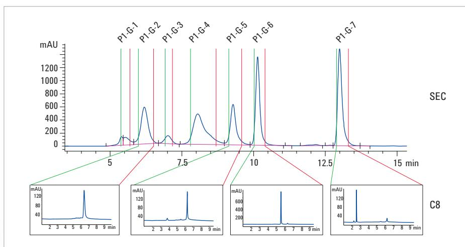
A re-analysis of the fractions confirms the exact fractionation procedure using peak-based fraction-trigger mode. The 2-position/6-port valve in the column compartment enabled automated column switching.
