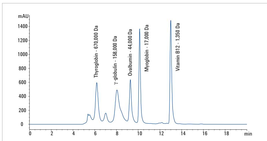
This gel filtration standard containing thyroglobulin,  $\gamma$ -globulin, ovalbumin, myoglobin, and Vitamin B12 was separated using SEC. Afterwards, we automatically collected the fractions (using peak-based fraction trigger mode) into ascertained wells of a deep-well plate. The fractions were then re-analyzed using a reversed-phase C8 column.
