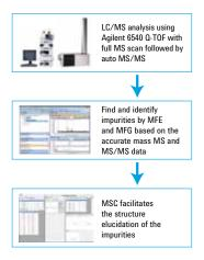
**Figure 5.** Software-assisted workflow for impurity identification and profiling of pharmaceuticals on the Agilent 1200 Infinity Series LC combined with an accurate mass Q-TOF, and MassHunter Qualitative Analysis and MSC software.<sup>7</sup>
