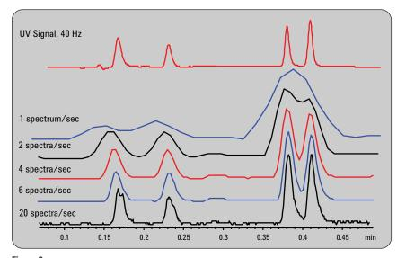
Figure 2 Effect of scan speed on resolution.
