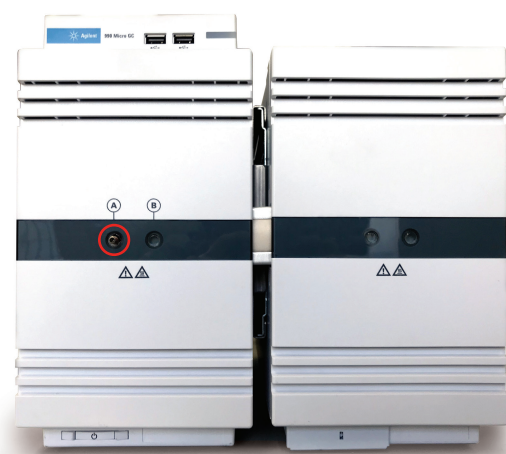
Figure 1B. Three-channel NGA analyzer. The red circle indicates the sample inlet.
