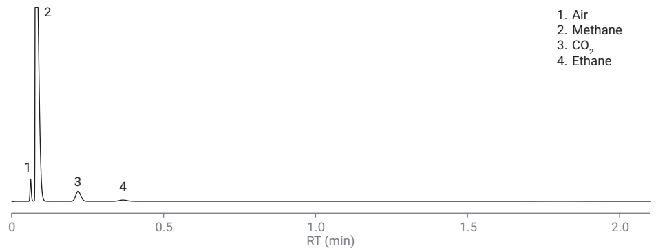
Figure 2A. Air, CO 2 , and C 1 to C 3 analysis on the HayeSep A straight channel.
