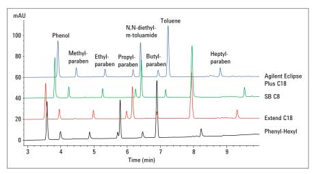
Figure 3. Overlay of chromatograms obtained from column scouting.
