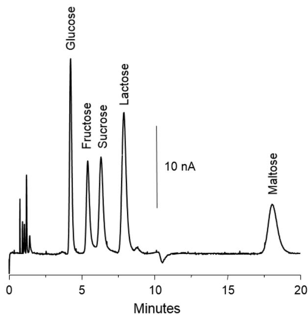
Fig. 28. Carbohydrate analysis in the pulse mode.
