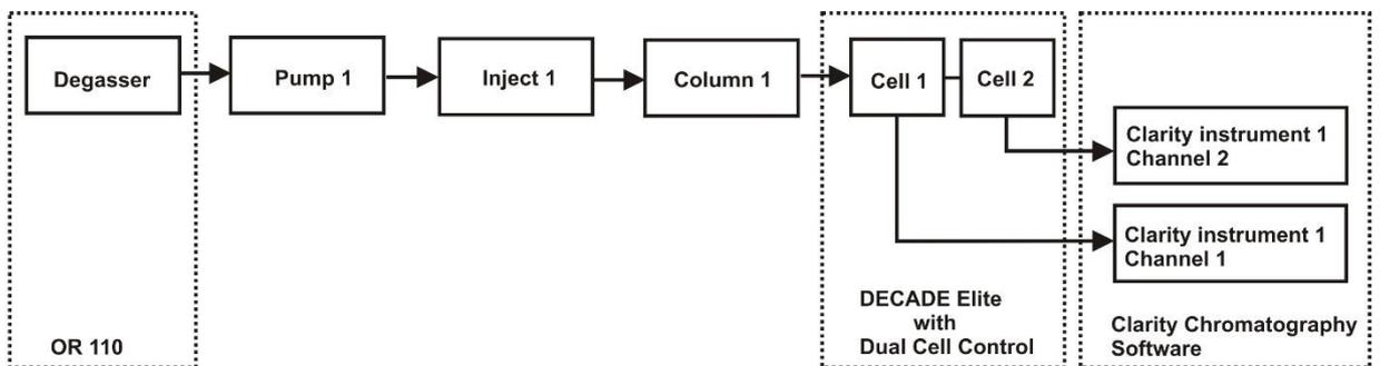
Fig. 11. Typical configuration for serial mode detection. Cell 1 is a FlexCell, cell 2 is a SenCell for detection. Channel 1 and 2 use the same time base of system 1.
