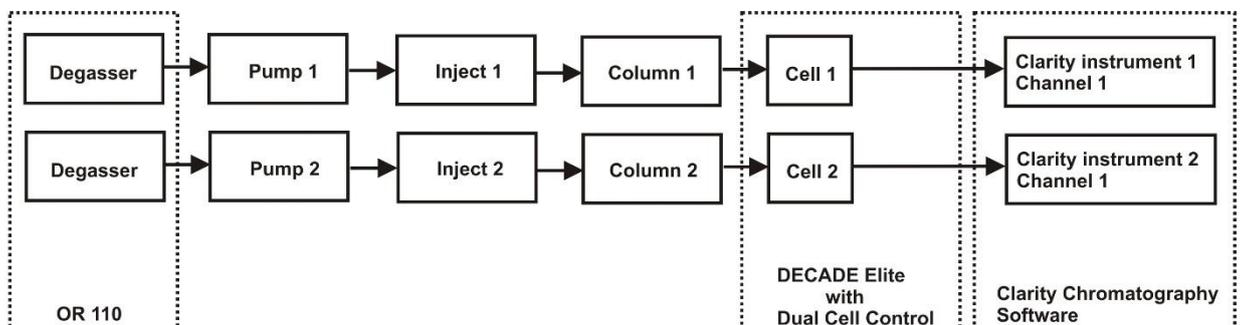
*Fig. 12. Typical configuration for parallel mode detection. Two independent HPLC systems with dual channel support from OR 110, DECADE Elite and Clarity software.*
