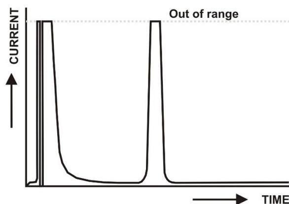
Fig. 47. Example of a chromatogram where the cell current exceeds the maximum current level and the signal is 'out of range'.
