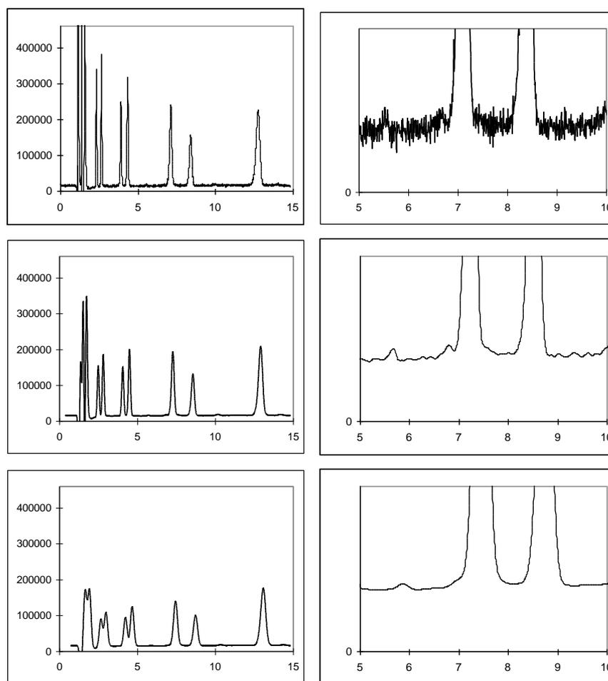
*Fig. 26. From top to bottom filter setting of 0.5, 0.02 and 0.002 Hz. Narrow peaks in front of the chromatogram are deformed at 0.005 Hz, whereas wider peaks show hardly any deformation (see peak at  $t \sim 13$  min). Attenuation of noise is shown in the close up on the right.*
