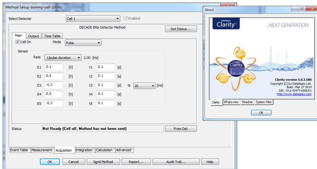
Fig. 8. DECADE Elite method window in Clarity. On the main tab the main measurement conditions can be set/controlled (measurement mode & potential settings).
