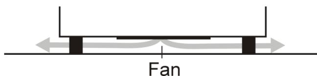
Fig. 2. Location of power supply fan DECADE Elite.
