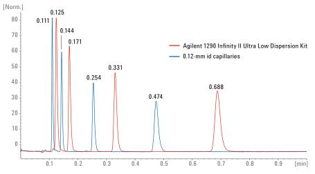
Figure 2. Isocratic separation of dimethylphthalate, diethylphthalate, biphenyl, and *o*-terphenyl using an Agilent 1290 Infinity II LC equipped with the Agilent 1290 Infinity II Ultra Low Dispersion Kit (red), and a standard Agilent 1290 Infinity II LC equipped with 0.12-mm id capillaries (blue).
