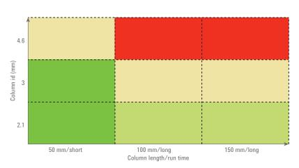
Figure 1. Overview improvements with ultralow dispersion kit for sub-2 µm particle columns (dark green – highly recommended, light green – highly recommend for isocratic runs, yellow – conditionally recommended, red – not recommended).
