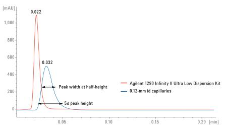
Figure 3. System dispersion measured at half-peak height and  $5\sigma$  for caffeine. The measured system dispersion was compared to a standard Agilent 1290 Infinity II LC equipped with 0.12-mm id capillaries, and to a system from another vendor.
