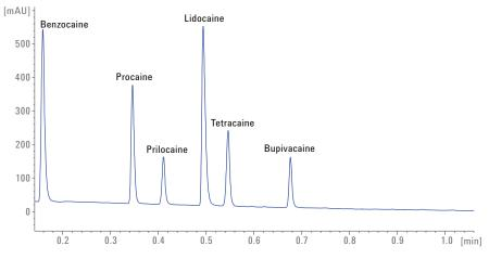
Figure 4. Gradient separation of six anesthetics using the Agilent 1290 Infinity II LC equipped with the Agilent 1290 Infinity II Ultra Low Dispersion Kit.
