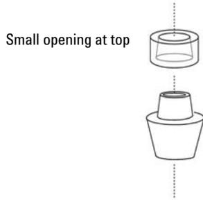
**Figure 7** Detail of PEEK ferrule and ferrule collar
