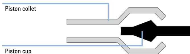
**Figure 10** Piston cup and piston collet
