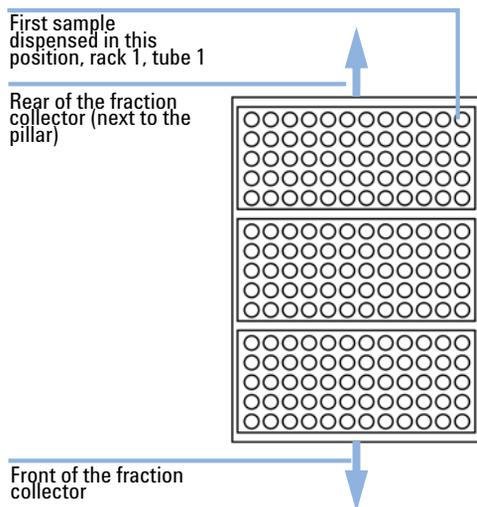
**Figure 21** Tube positions on the fraction collector
