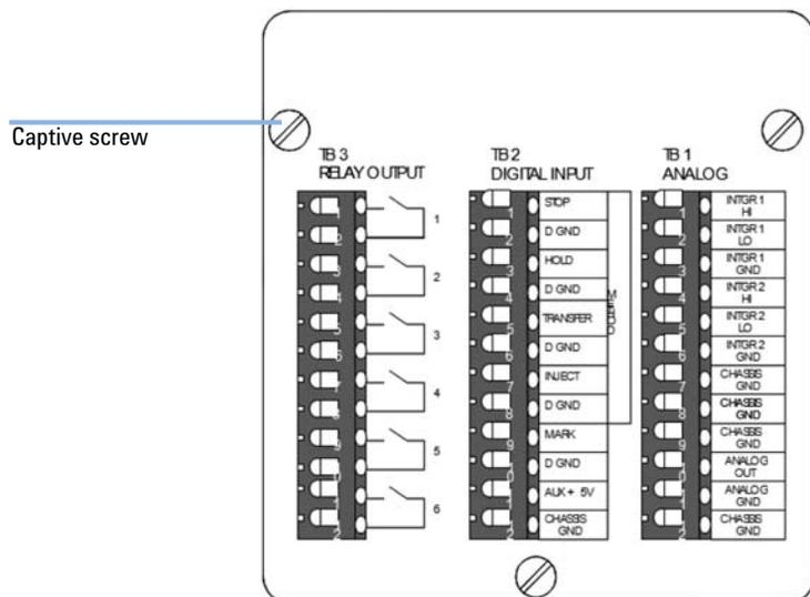
**Figure 5** External contacts panel (panel turned 90° for clarity)
