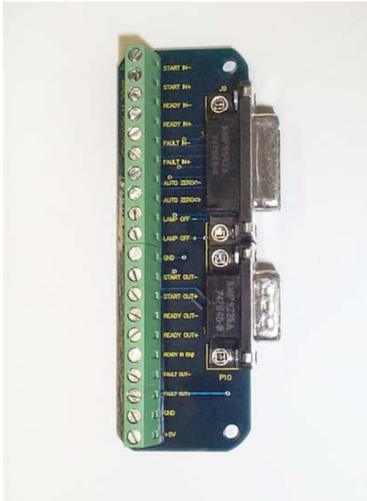
**Figure 29** The I/O adapter board
