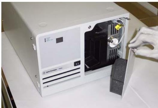
**Figure 13** Removing the front panel
