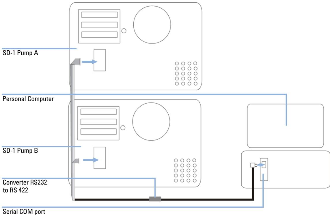
Figure 6 Connections for instrument control software (IBM/PC compatible)
