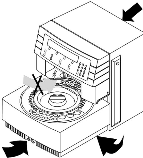
**Figure 1** Agilent 410 Autosampler lifting instructions
