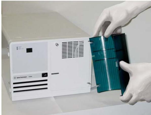
**Figure 15** Installing the Agilent 325 Detector door
