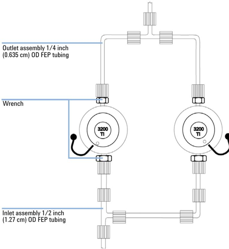
**Figure 8** Connections for 3.2 L pump heads
