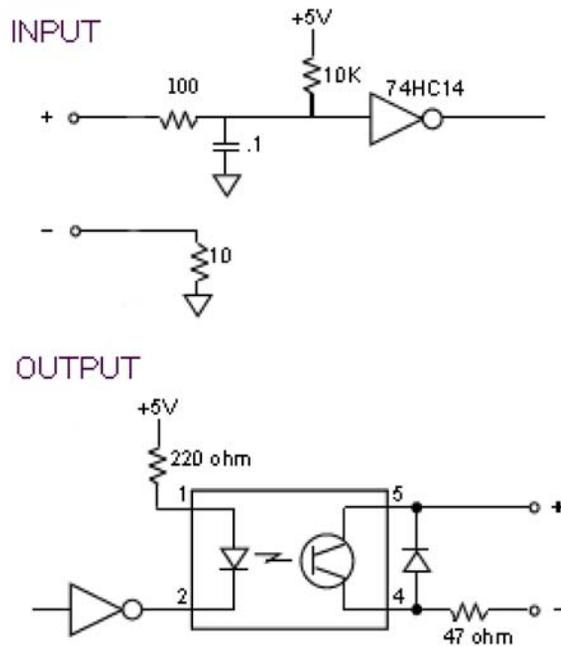
**Figure 28** Input/output schematics
