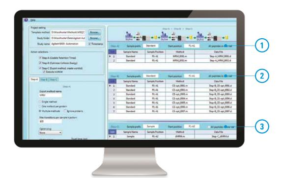
The Agilent Automation tool allows the user to select the steps and parameters for MRM method development.
