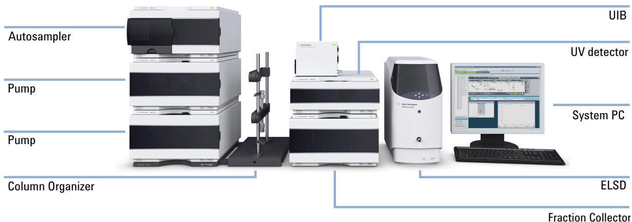
Figure 6 Configuration of a 1260 Infinity Series Purification System with ELSD
