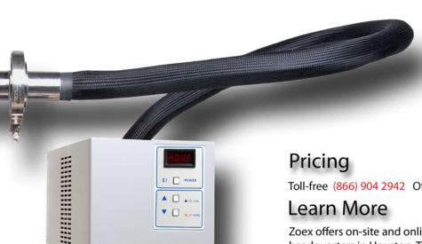
Continous cooling without liquid nitrogen Maximum cooling temperature: -90°C at the jet SS vacuum insulated cold gas delivery line 30" long :316 corrugated stainless Cooling Probe Refrigerant expands directly inside the probe Compressor :2 compressors @ 1/4 hp Dimensions :10" x 20" x 18.5"
